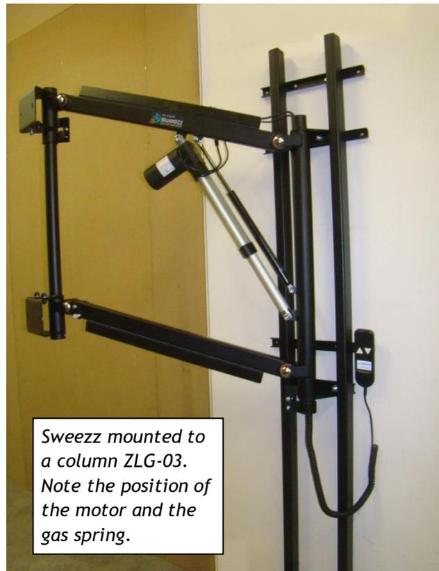
**Important:** There is a new motor: a high quality TiMOTION actuator is provided with the Sweezz. This actuator has to be mounted with the electrical motor part upwards, as in this picture (this differs from older versions). The gas absorber/spring must have the thin end up.
